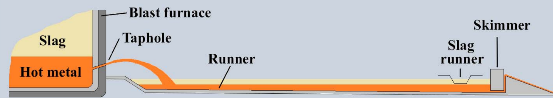
Figure: Blast furnace runner schematic diagram.
