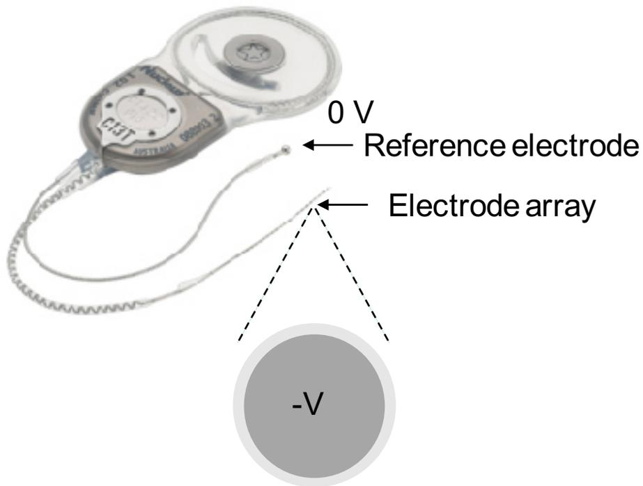
Standard electrode:  $\approx$  disc at -V volts
