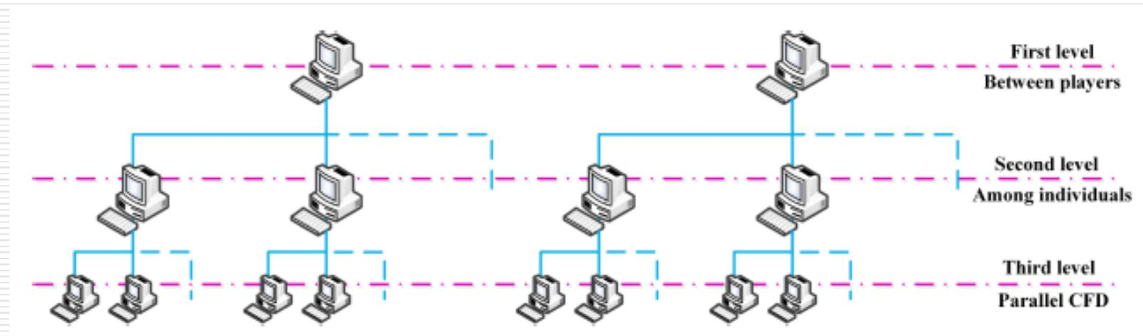
Diagram showing the three levels of parallelism implemented in *Nash Evolutionary Computing*.
