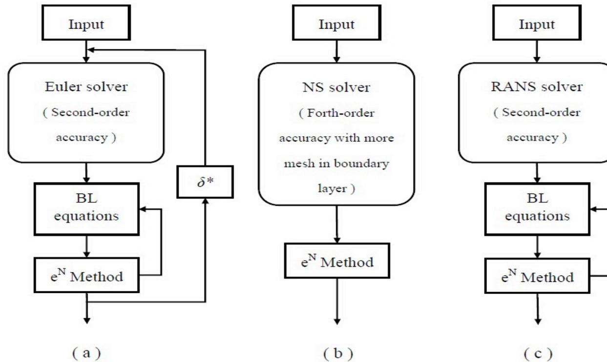
Three flow charts of the coupling between flow field solver and transition prediction
