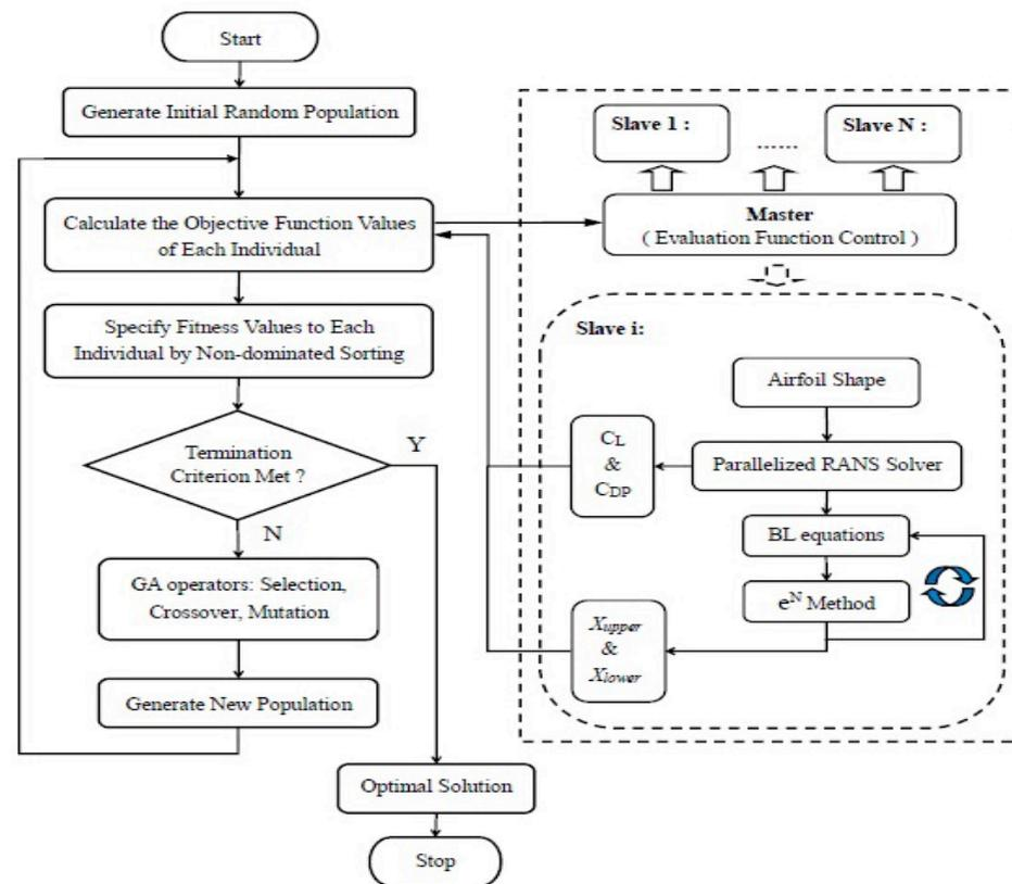
Flow chart of a parallelized NSGA-II optimization procedure for a laminar flow airfoil shape optimization.
