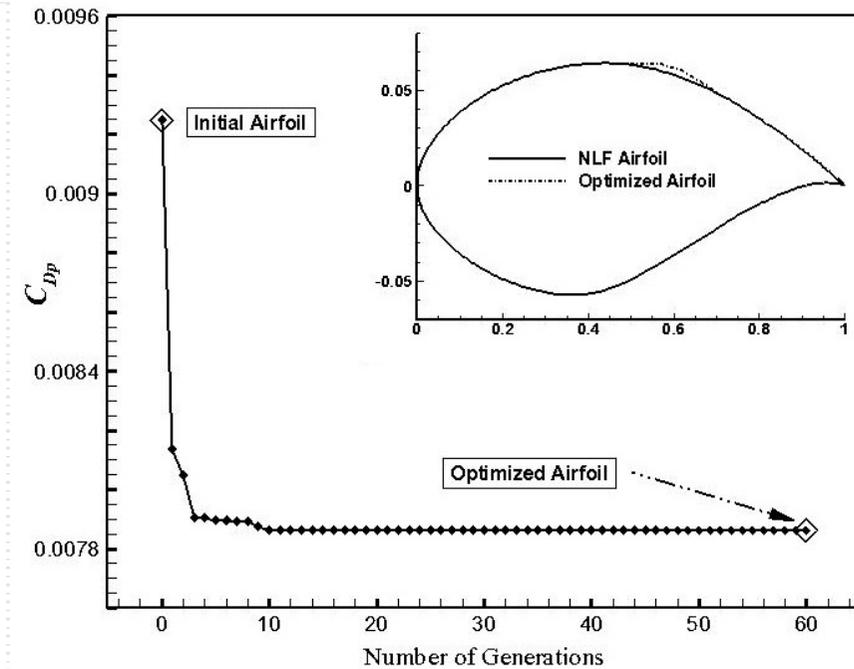
Convergence history for shape optimization of a bump installed on the RAE2822 airfoil ( left ) and the NLF airfoil ( right ).
