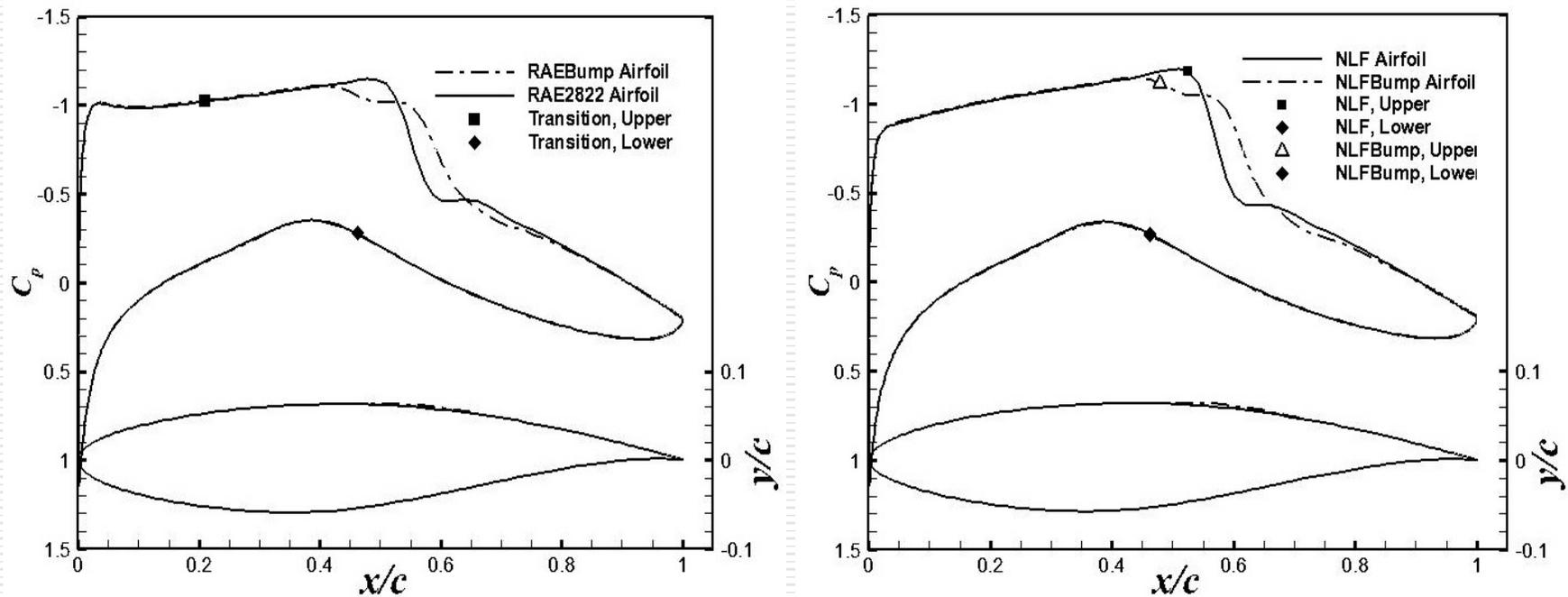
Results : Pressure distributions and transition locations on RAE2822 airfoil and airfoil equipped with a bump ( left ) and on NLF airfoil equipped with a bump ( right ).
