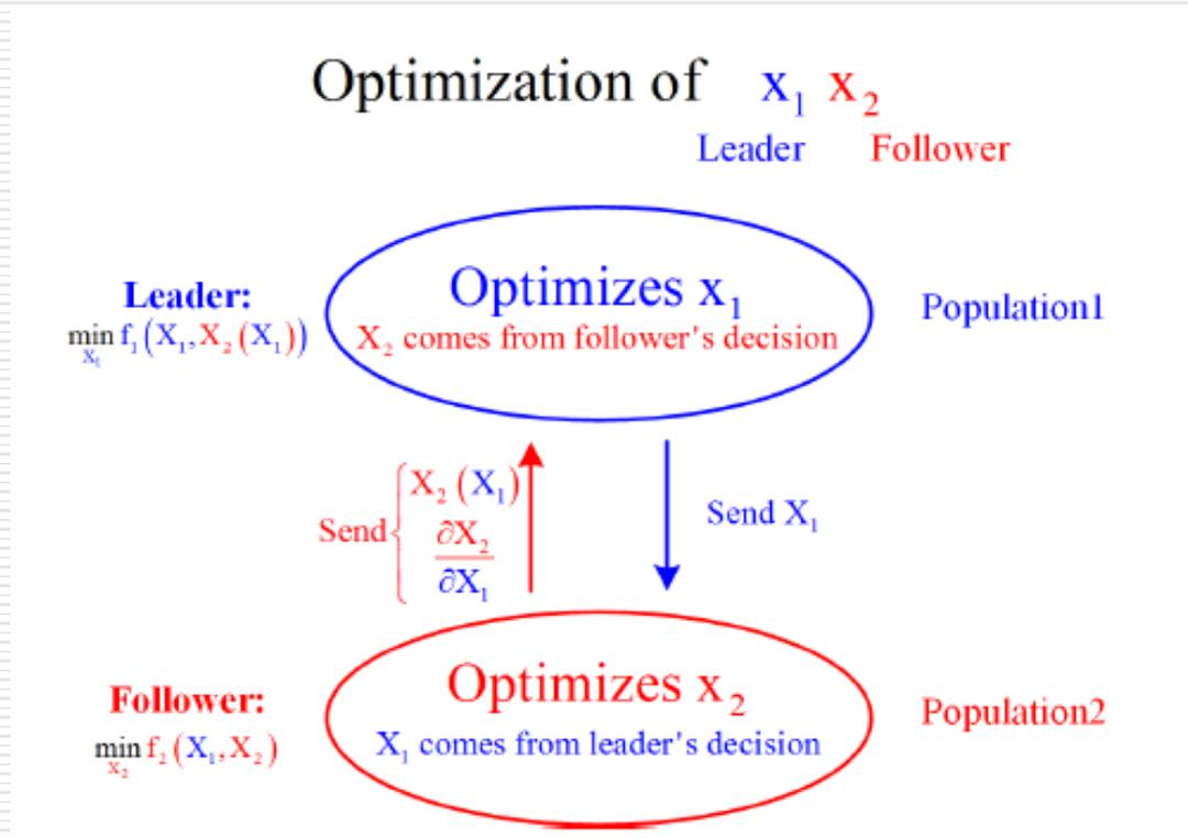
*Diagram of a Stackelberg Evolutionary Algorithm.*
