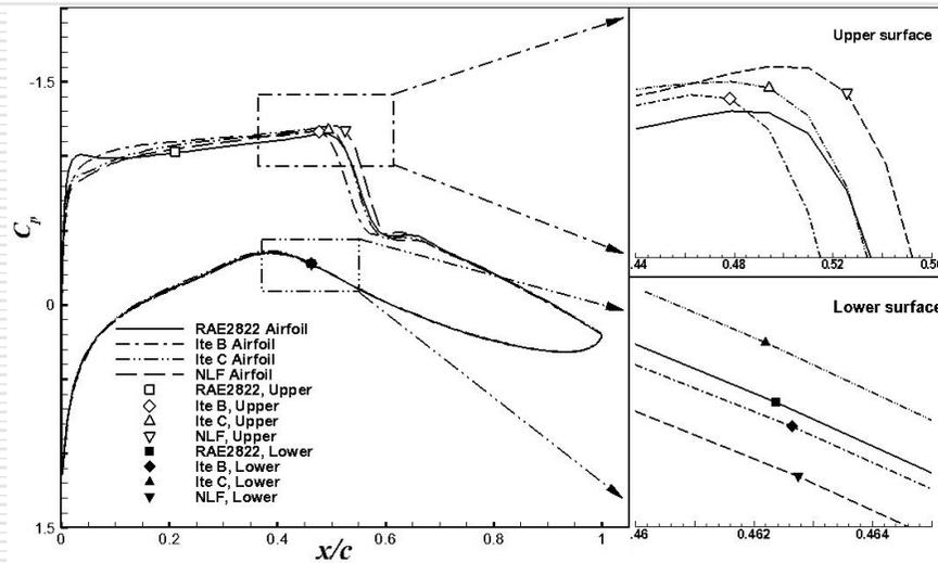
*The laminar flow range increased, but **the wave strength increased simultaneously!***
