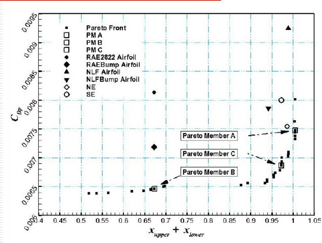
**Fig.1** Converged Pareto front and solutions of NE, SE, RAE Bump, NLF, NLF Bump and Baseline shape.
