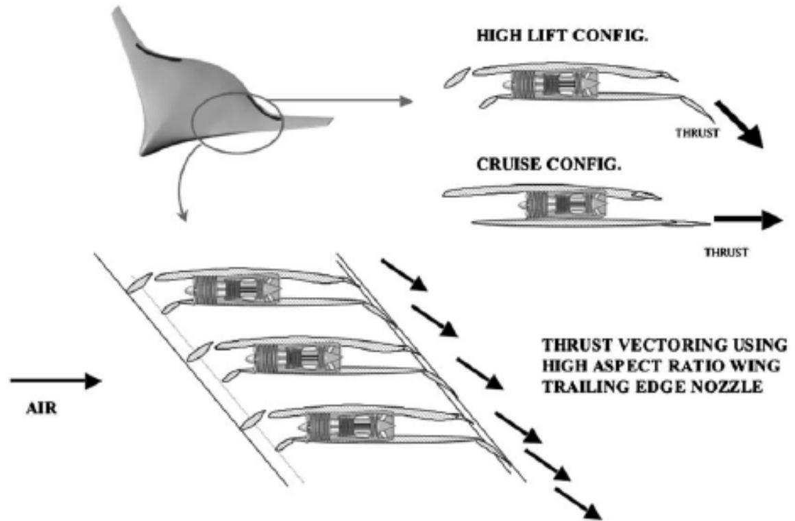
**Distributed engines embedded in blended wing body aircraft**
