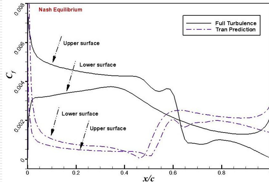
Comparison of skin friction coefficient distributions between full turbulence simulation and simulation with transition prediction on
