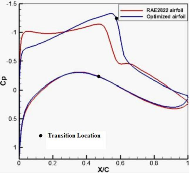
*But the larger the region of laminar flow is, the stronger the shock wave is ! (compare figures 1-2-3)*
